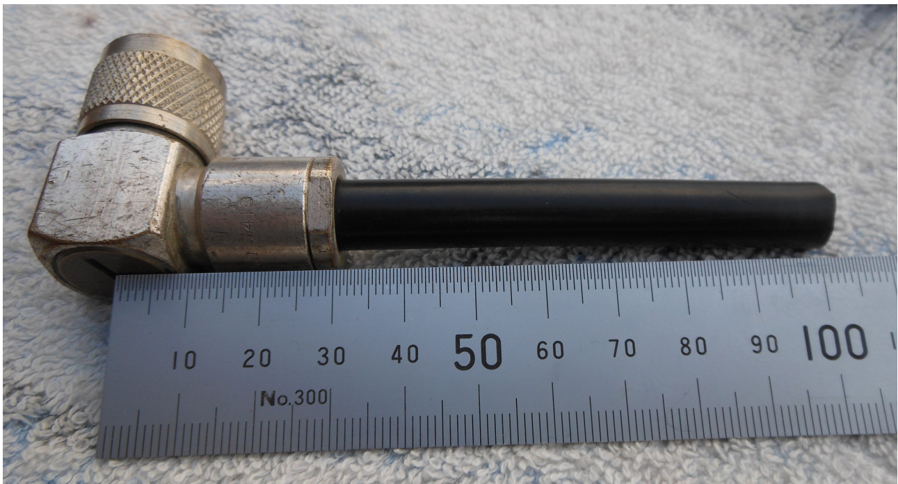
Picture-2. Tuning open circuit stub 105 mm to centre of elbow.
