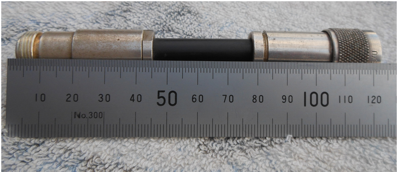
Picture-1. Matching section 123 mm connector tip to tip.
