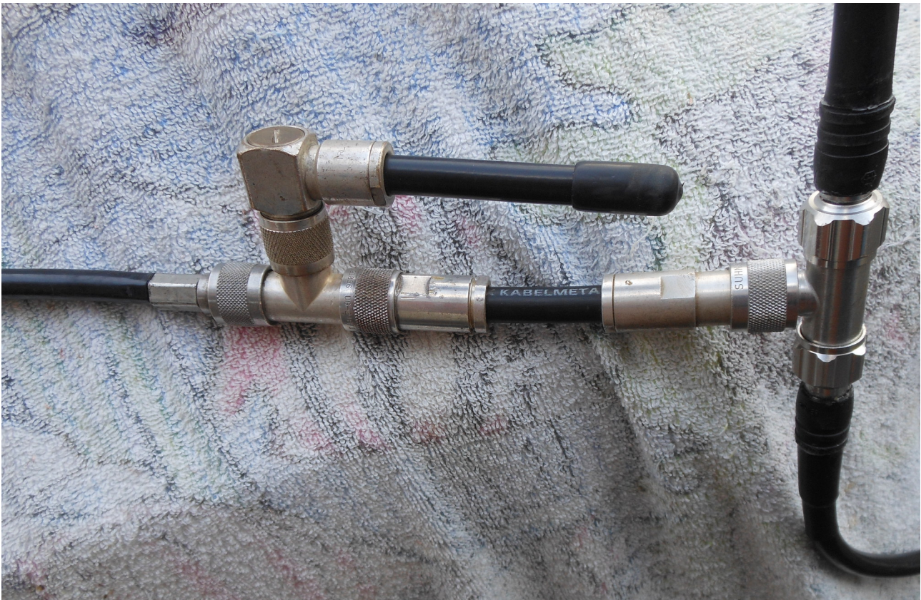
Picture-3. Both dipoles connected and return loss of -23.5 db measured without 8 m feeder cable.
